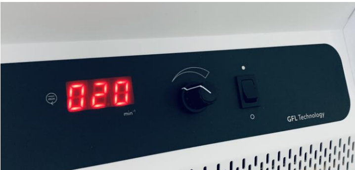
Control panel for setting and display of the shaking frequency H 20 SW und H 20 SOW
